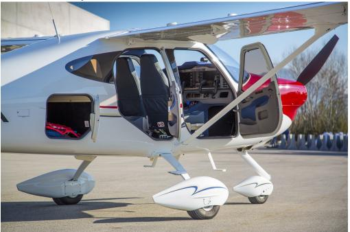
This four-seater aeroplane brings together an advanced technology all carbon fibre fuselage with a metal wing and stabilator, an expansive cabin featuring ergonomic front and rear seats with exceptional legroom and a separate third entry door.
